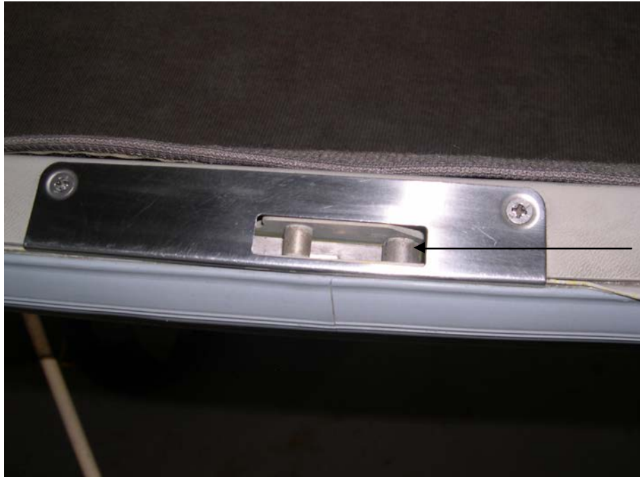
Door not locked switch on key lock
