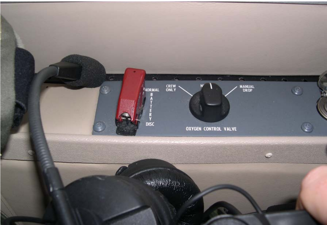
Oxygen Control Panel, left armrest
