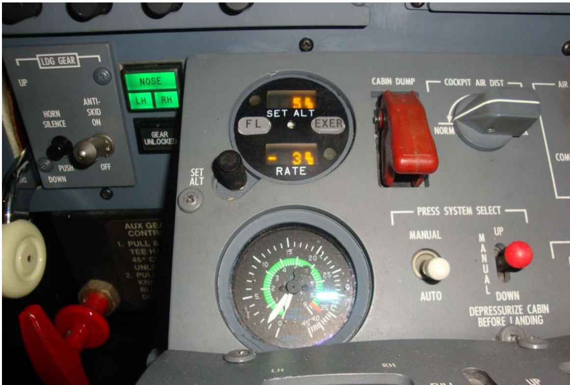
Pressurization Tilt Panel. Note “SET ALT” knob
