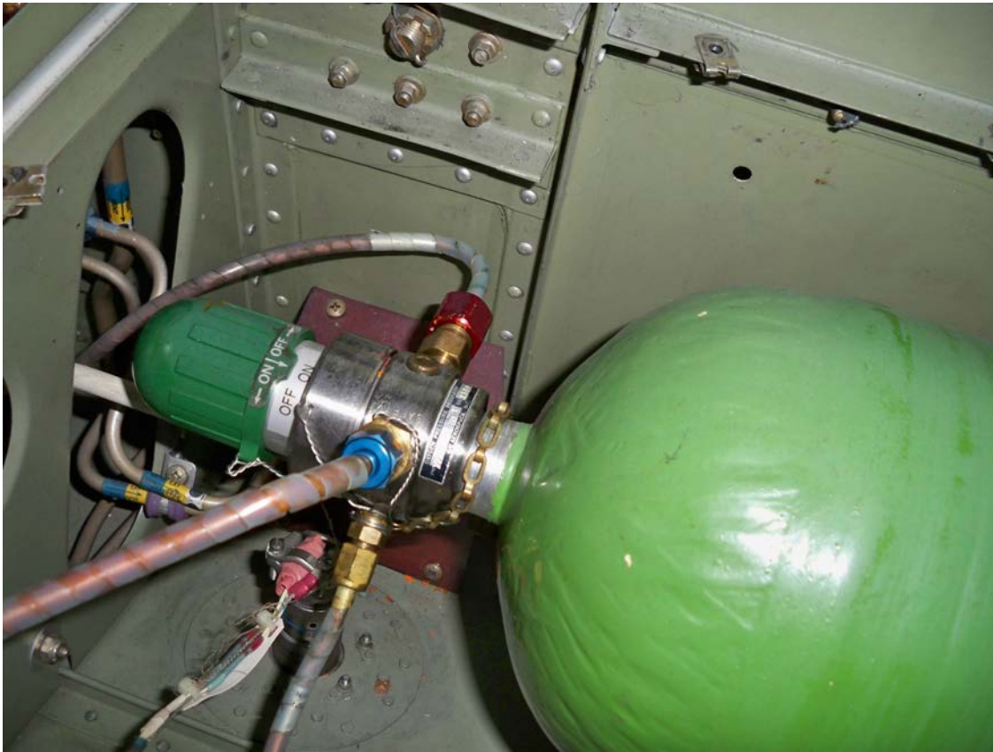
Oxygen Bottle mounted in the nose
