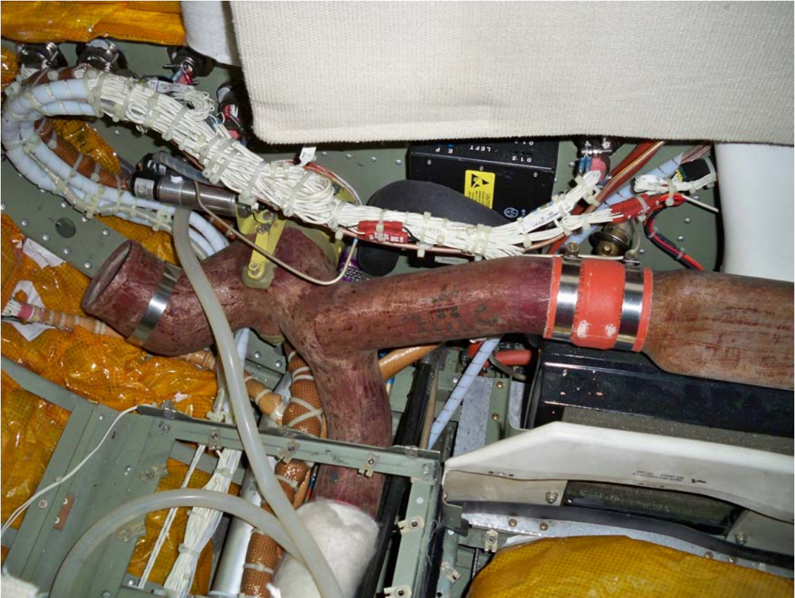
The photo above shows the possible paths incoming environmental air can flow through.
