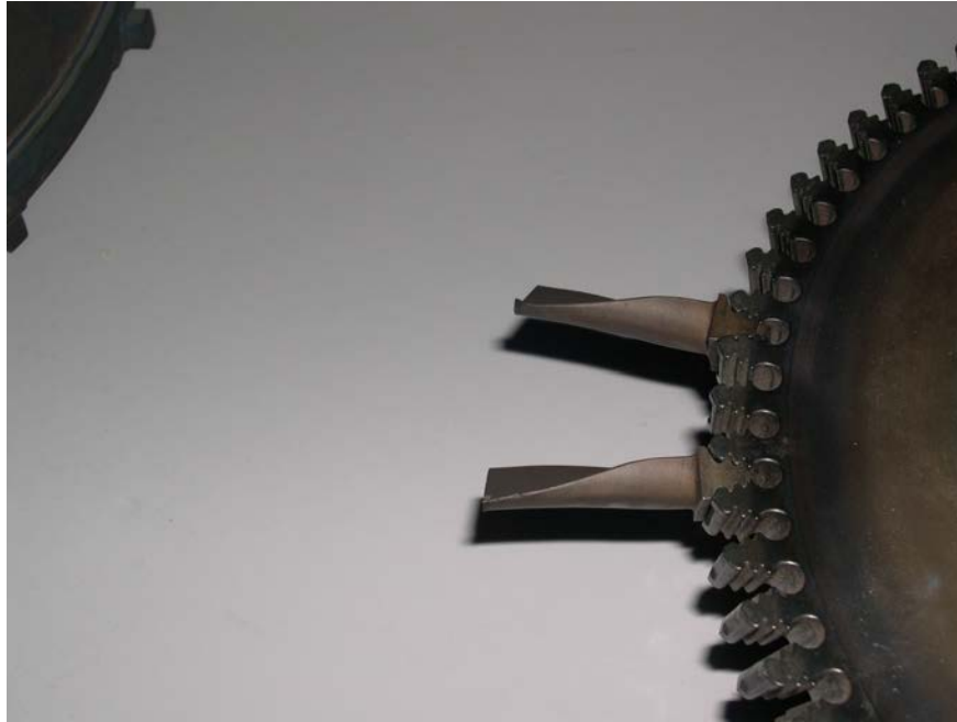
High Turbine Disk with 2 blades inserted
